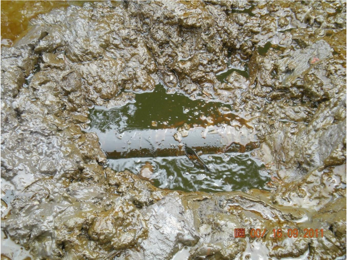
Close-up: Spill due to hack saw cut on Akaso Well 10S flowline at Mbiana. Picture was taken during Joint Investigation of 16th September, 2011.
