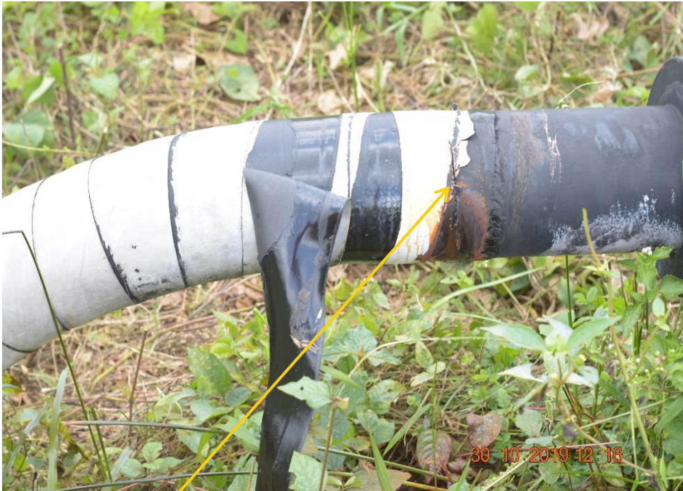
Close-up: Hack Saw Cuts on 4" Agbada2 Well 58 Flowline at Omueke. Picture was taken during Joint Investigation of 30 th October 2019.
