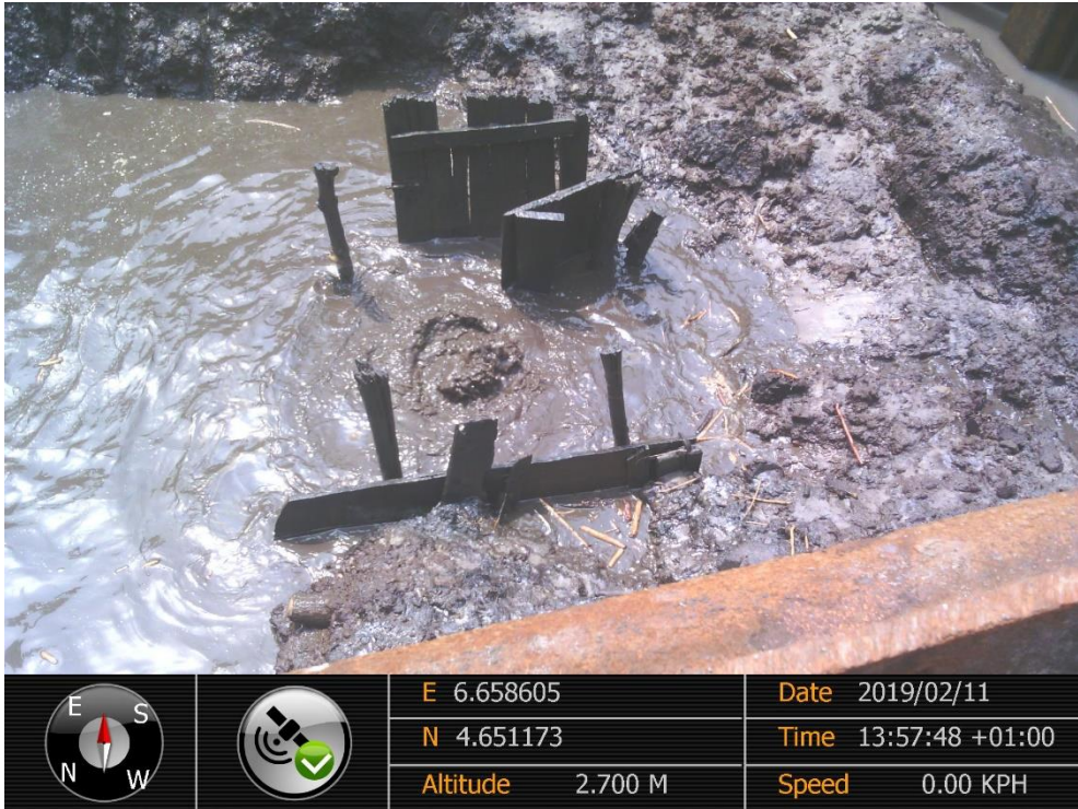
Overview: Part of spill impact on 18" Soku – Buguma Pipeline Right of Way at Soku. Picture was taken during Joint Investigation of 11 th February 2019.
