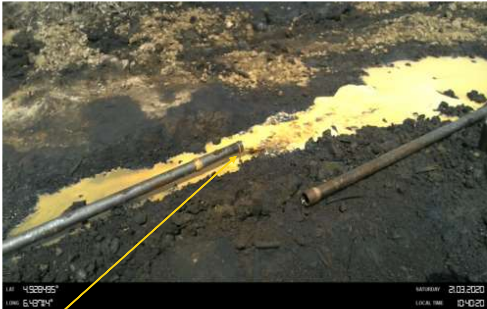
Close-up: Crude oil theft points at 12 o'clock position on Old 20" Kolocreek – Rumuekpe Pipeline at Odau. Picture was taken during Joint Investigation of 21 st March 2020.
