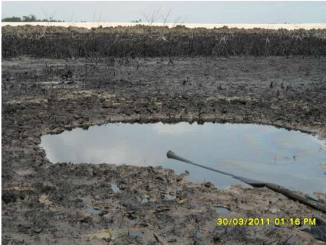
Overview: Extent of the spill incident impact on 24in Bomu-Bonny pipeline at Bodowest. Spill site showing oil theft hose still attached to illegal off take point.
