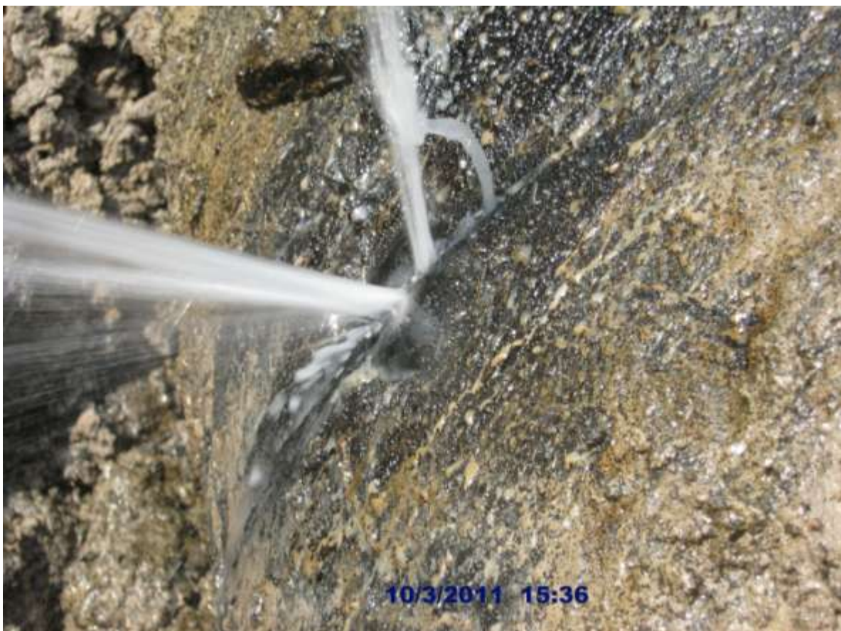
Close-up: Hacksaw cut on 24' Bomu-Bonny Pipeline at Moghor. Picture was taken during JIV of 10 March 2011
