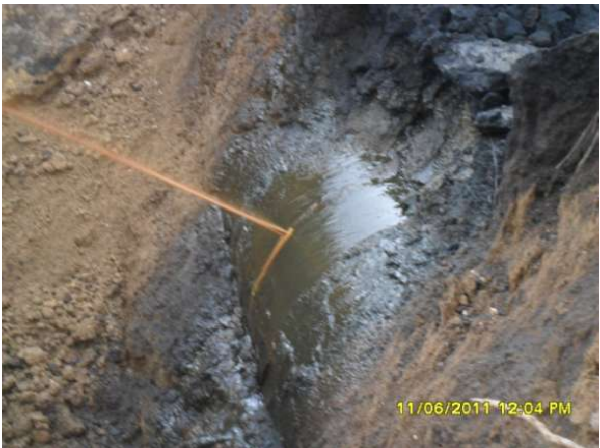
Close-up: Spill due to cut on 28'' Bomu- Bonny Pipeline at Bodo (Ogoni). Picture taken during Joint Investigation of 11 th June, 2011.
