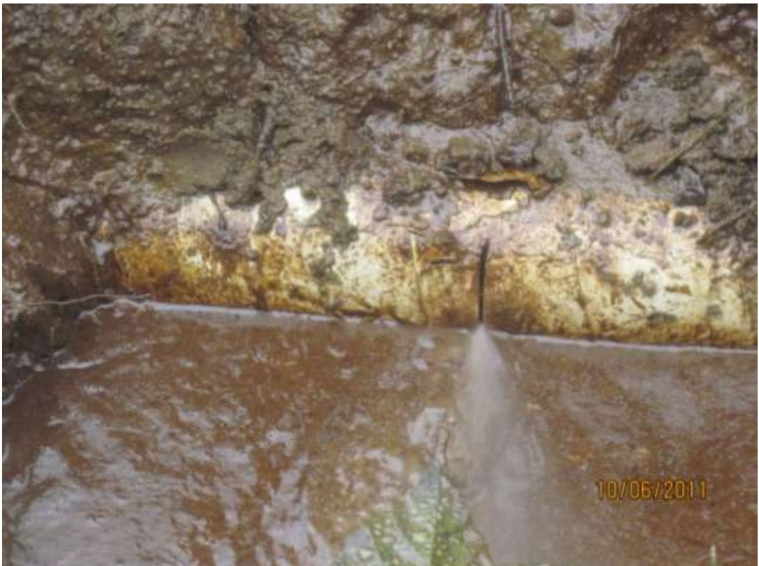
Close-up: Hacksaw cut on Obigbo Well 28LS flowline at Imea. Picture taken during Joint Investigation of 10 th June, 2011
