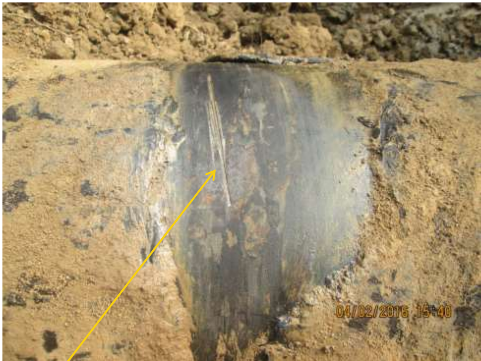
Close-up: Hacksaw cut on 16" Nun River – KoloCreek Pipeline at Aguobiri. Picture was taken during Joint Investigation of 4 th February 2016.
