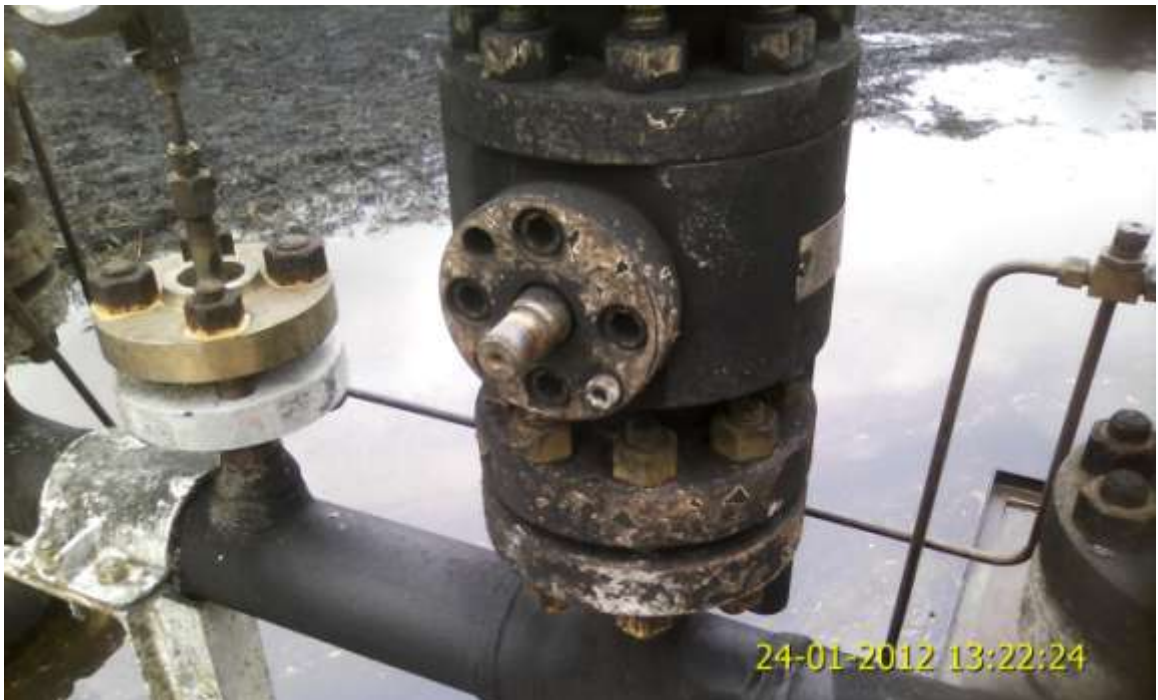
Close-up: Tampered valve on Etelebou Well11 at Akenfa-Epie. Picture was taken during Joint Investigation of 24 th January 2012.
