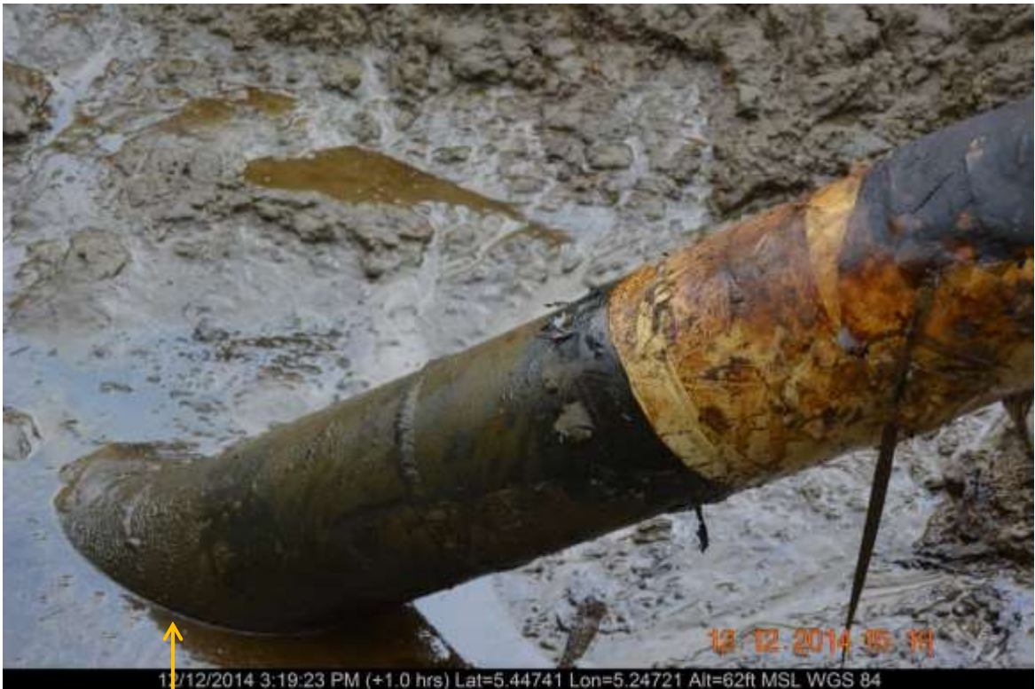
Close-up: Spill due to pinhole leak on 6" Yokri Manifold8 Test Flowline at Yokri. Picture was taken during Joint Investigation of 12 th December 2014.
