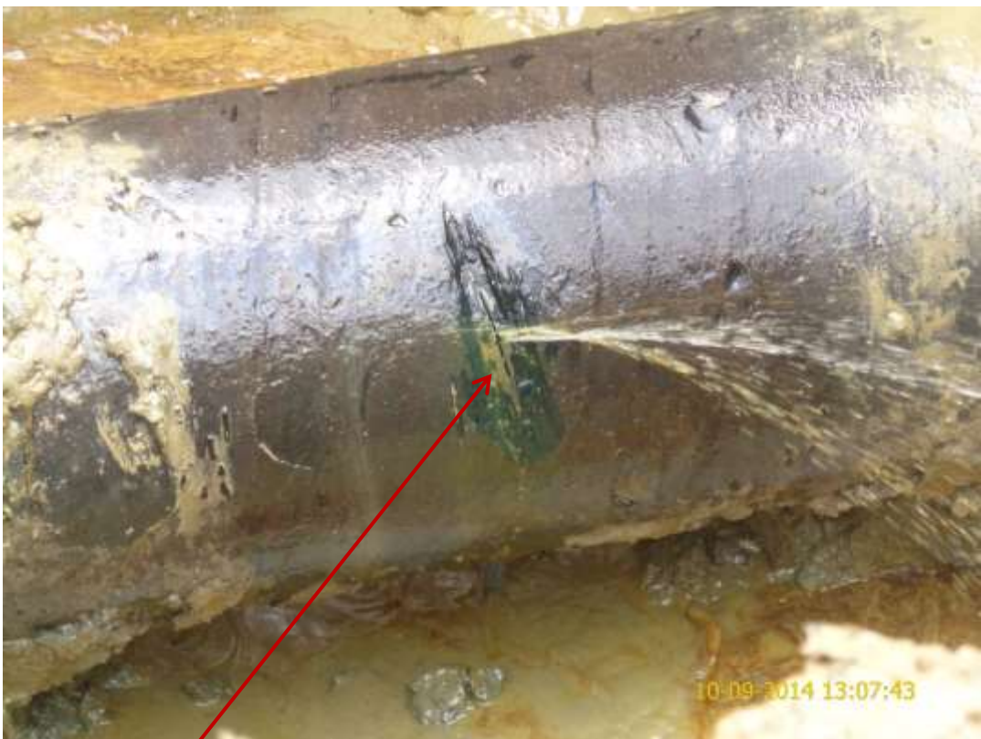
Close-up: Hacksaw cut on 10" Diebu Creek – Nun River Pipeline Right of Way at Ekowe. Picture was taken during Joint Investigation of 10 th September 2014.
