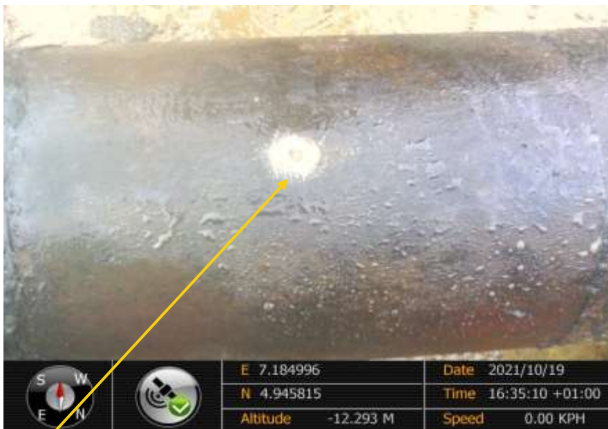
Overview: Part of spill impact on 12" Imo river 1- Ogale Pipeline at Umulolo. Picture was taken during Joint Investigation of 19 th October 2021.
