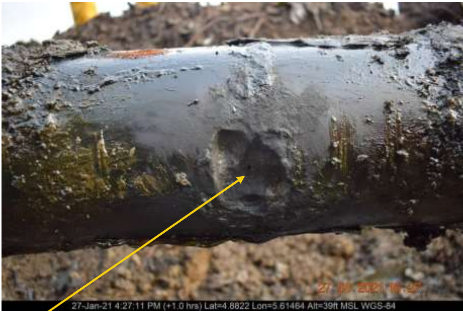
Overview: Part of spill impact on 6inch kanbo well 6T flowline at Tunu . Picture was taken during Joint Investigation of 27 th January 2021 .
