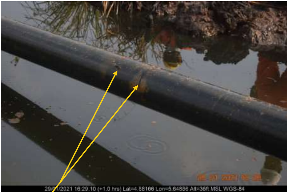
Overview: Part of spill impact on 6inch Kanbo Well 7s flowline at Agbidiama. Picture was taken during Joint Investigation of 29 th January 2021.
