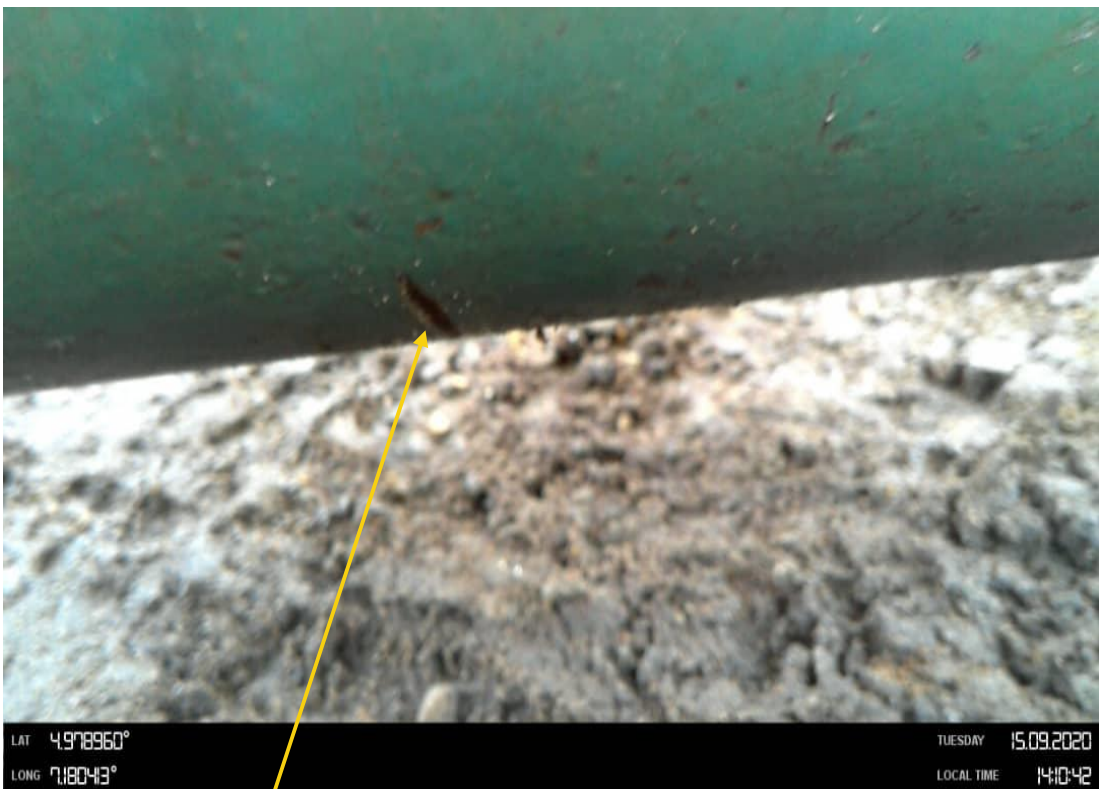
Close-up: 72mm Hacksaw cut at 5 to 6 o'clock position on Imo River 1 Well 44s Flowline at Igiriukwu Isi-Etithoha. Picture was taken during Joint Investigation on 15th September 2020.
