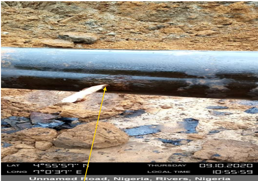
Close-up: Plugged rough edge tear at 9 o'clock position on 8" Agbada 2 Nkpoku DeliveryLine at Omuohia - Igwuruta. Picture was taken during Joint Investigation on 10th September 2020.
