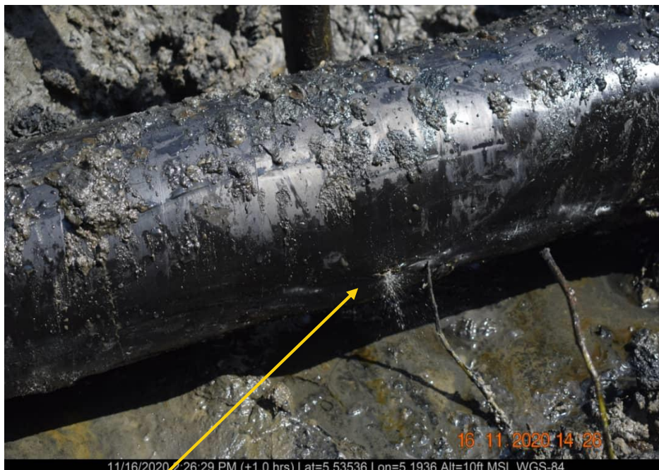
Close-up: Tear at 3 o'clock position on 6inch Escravos Well 13s Flowline at Ogidegben. Picture was taken during Joint Investigation on 16th November 2020.
