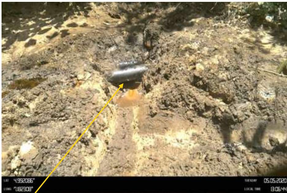
Close-up: Hacksaw cut at 6 o'clock position on 4" ImoRiver Well 55s Flowline at Igiriukwu. Picture was taken during Joint Investigation 5th May 2020.
