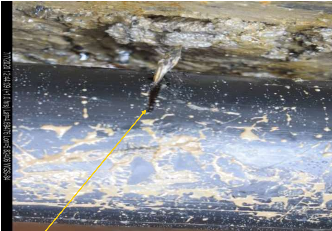
Closeup 2: Hack saw cut at 3'o clock position and 9 o'clock position on 8" Seibou-Ajatiton Bulklineat Agbidiaama. Picture was taken during Joint Investigation 7th July 2020.
