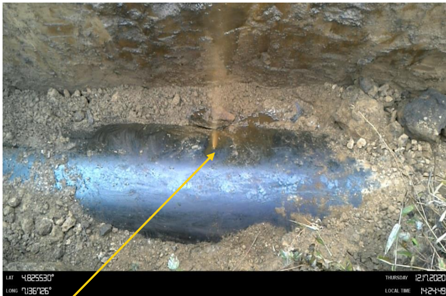
Close-up 3: 4 nos 5mm drilled hole (leak point 2) at 1 o'clock position on 36inch Nkpoku Ogale Pipeline at Agbonchia. Picture was taken during Joint Investigation on 17th Dec 2020.
