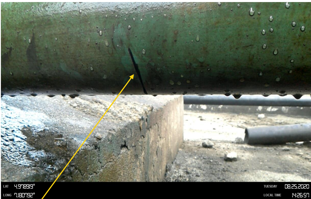
Close-up: 4cm Hacksaw cut at 5 to 6 o'clock position on 4" ImoRiver 1 well 36s Flowline at Isietitioha Owaza. Picture was taken during Joint Investigation on 25th August 2020.
