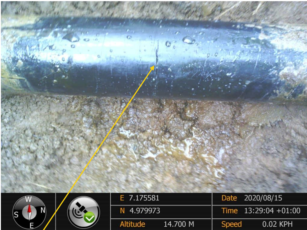
Close-up: Hack Saw Cut at 1 o'clock to 5 o'clock position on 4" Imo River2 – Imo River1 Bulcline at Igiriukwu - Isietitiuzo -Owaza. Picture was taken during Joint Investigation of 15 th August 2020.
