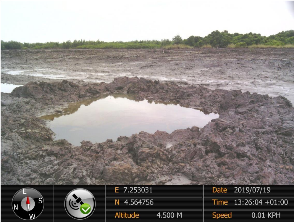
Overview: Part of spill impact on 24" Bomu – Bonny Pipeline Right of Way at Owokiri. Picture was taken during Joint Investigation of 19 th July 2019.
