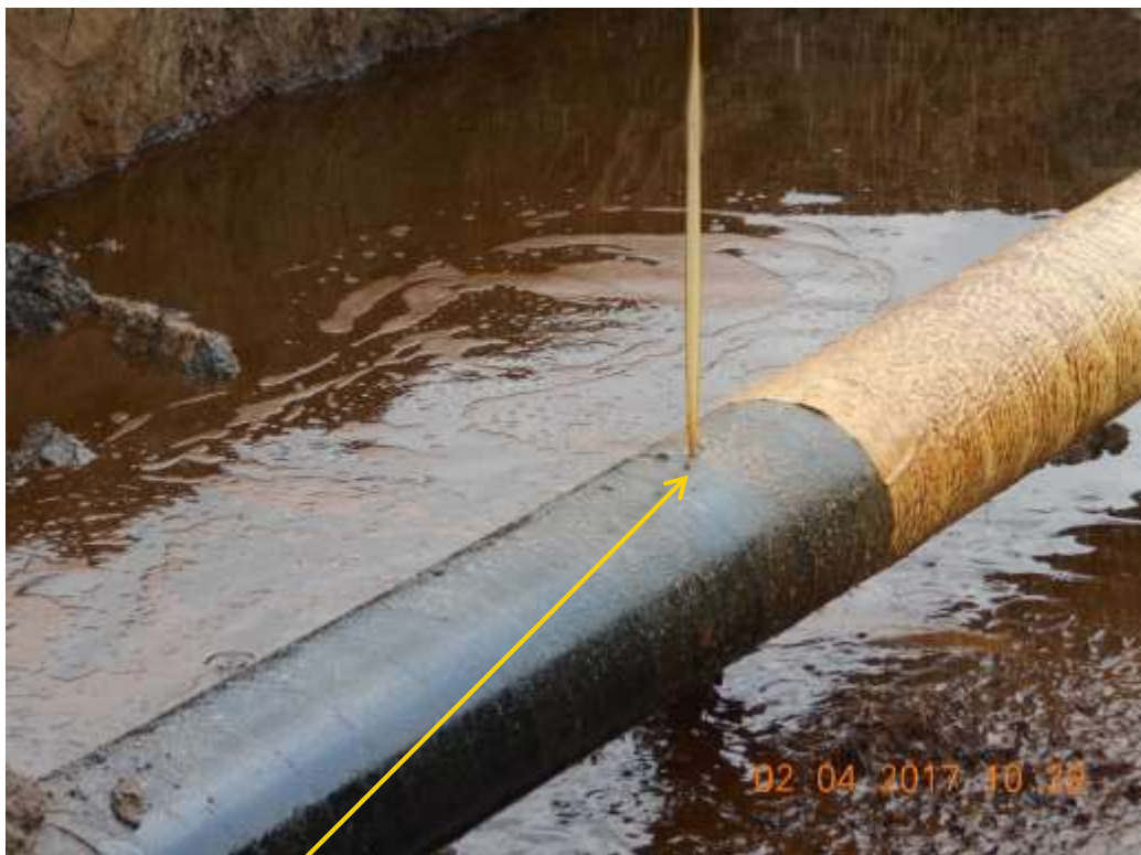
Close-up: Drilled hole on 12" Imo River – Ogale Pipeline at Uzuaku Picture was taken during Joint Investigation of 2 nd April 2017.
