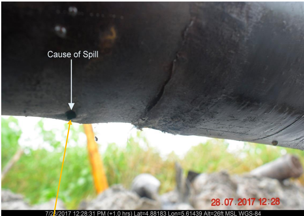
Overview: Part of spill impact on 4" Tunu Well-4L Flowline at Agbidiana. Picture was taken during Joint Investigation of 28 th July 2017.
