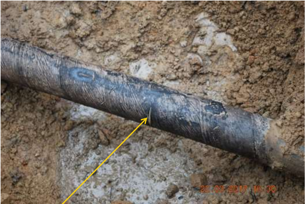
Close-up: 4 th of 5 Hacksaw cuts on 4" Obele-Ibaa Pipeline at Ibaa. Picture was taken during Joint Investigation of 22 nd March 2017.
