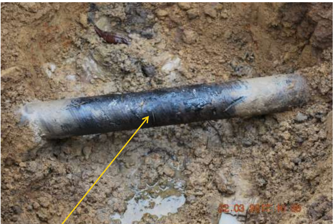
Close-up: 5 th of 5 Hacksaw cuts on 4" Obele-Ibaa Pipeline at Ibaa. Picture was taken during Joint Investigation of 22 nd March 2017.
