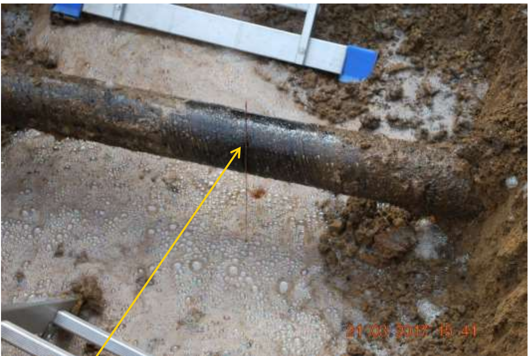
Close-up: 3 rd of 5 Hacksaw cuts on 4" Obele-Ibaa Pipeline at Ibaa. Picture was taken during Joint Investigation of 21 st March 2017.
