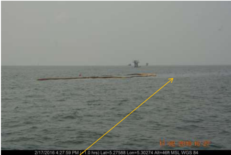
Overview: Containment boom and oil slick observed around the leak point on 48" Forcados Terminal Export Line. Picture was taken during Joint Investigation of 17 th February 2016.
