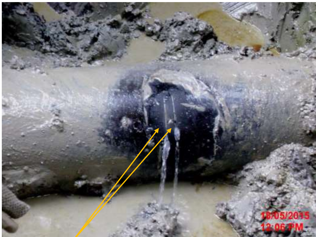
Close-up: Hacksaw cuts on 10" Diebu Creek – Nun River Pipeline at Oporoma. Picture was taken during Joint Investigation of 18 th May 2015.
