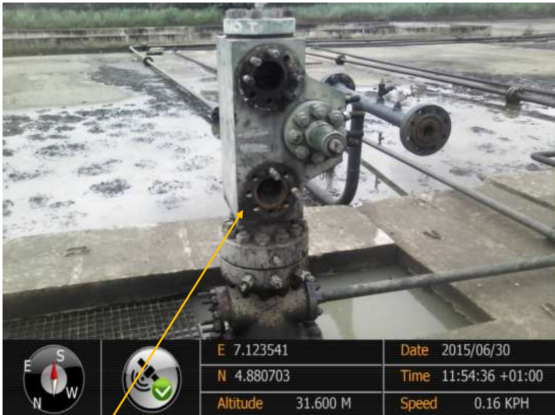
Close-up: Tampered wellhead on Obigbo Well10T Wellhead at Umudinor. Picture was taken during Joint Investigation of 30 th June 2015.
