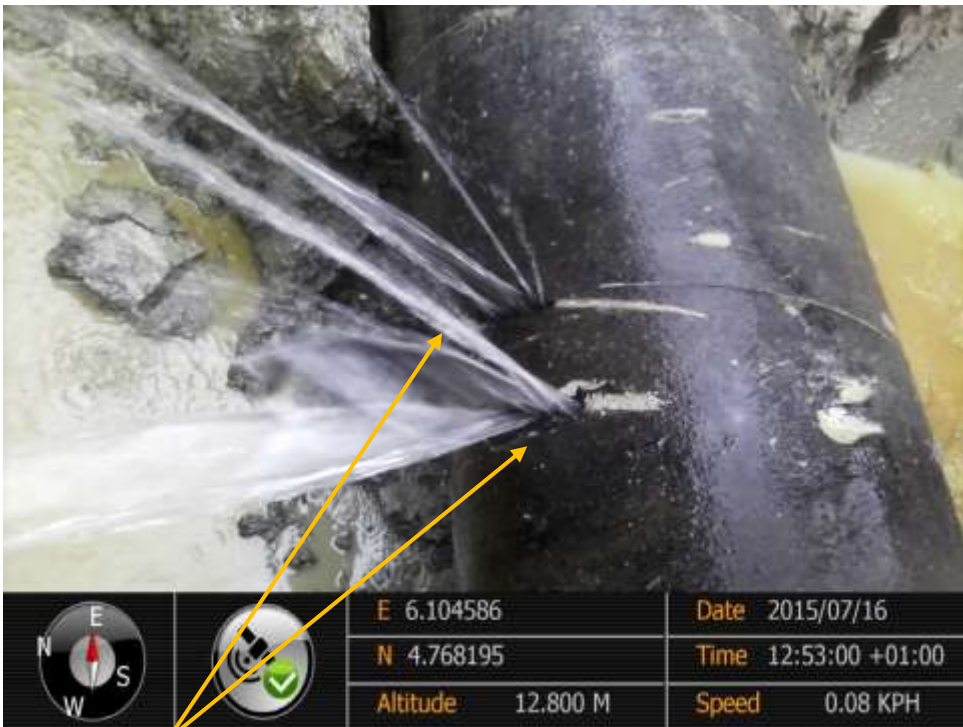
Close-up: Hacksaw cuts on 10" Diebu Creek – Nun River Pipeline at Oporoma. Picture was taken during Joint Investigation of 16 th July 2015.
