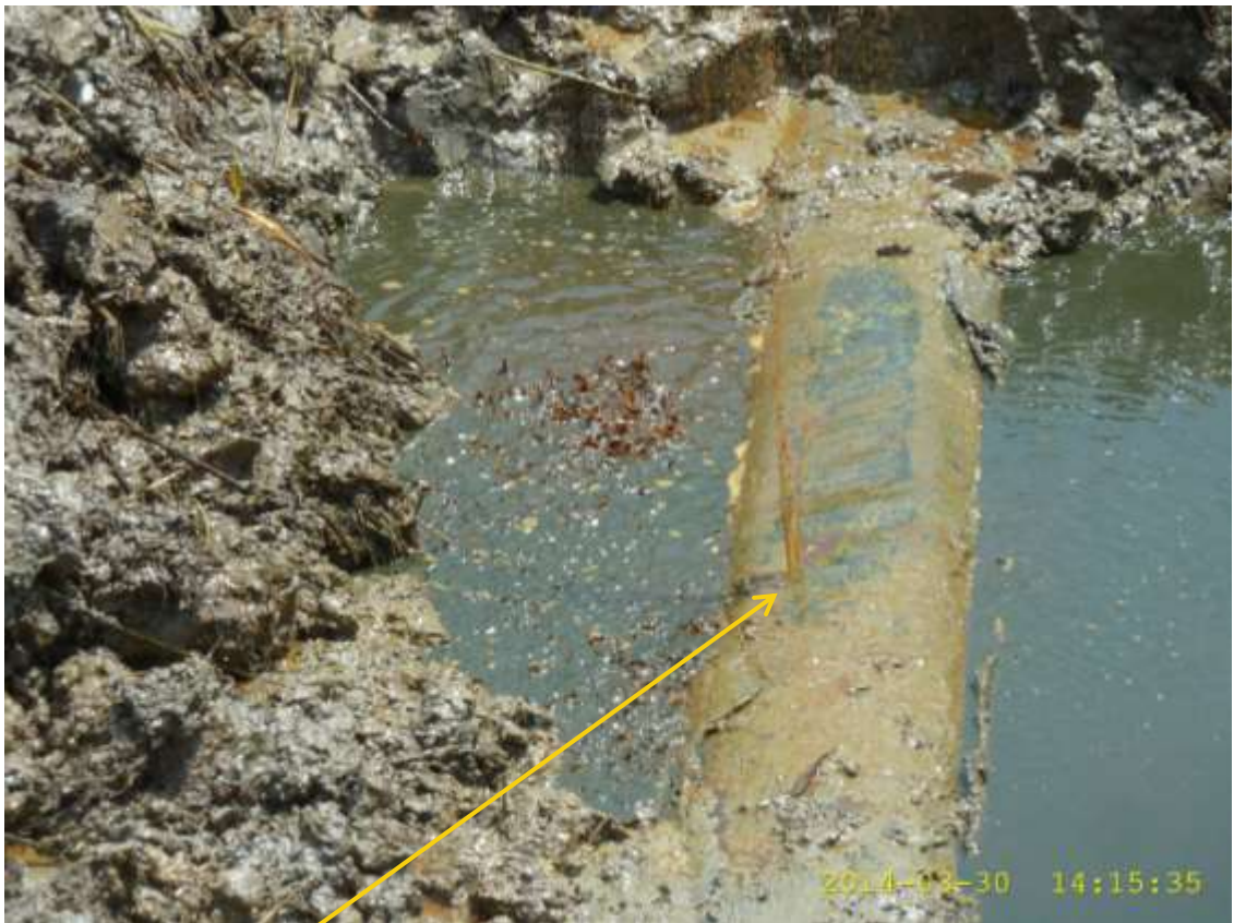
Close-up: Spill due to tear on 10" Diebu Creek Manifold – Nun River manifold at Peremabiri. Picture was taken during Joint Investigation of 30 th March 2014.
