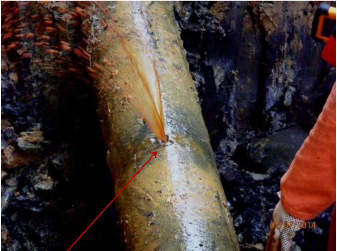
Close-up: Spill Point2, 95.5m from Spill Point1, on 10" Diebu Creek – Nun River Pipeline at Onyoma/Enewari. Picture was taken during Joint Investigation of 3 rd July 2014
