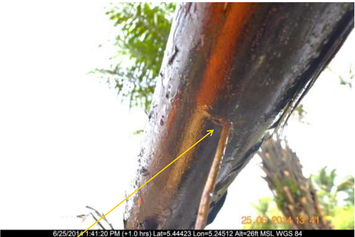
Close-up: Spill due to corrosion on Yokri Well 110T Flowline at Yokri. Picture was taken during Joint Investigation of 25 th June 2014.
