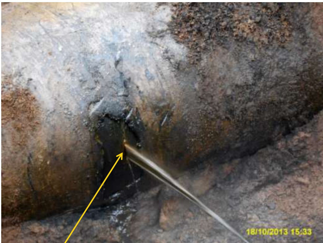
Close-up: Hacksaw cut on 24" Nkpoku - Bomu Pipeline at Biara. Picture was taken during Joint Investigation of 18 th October 2013.
