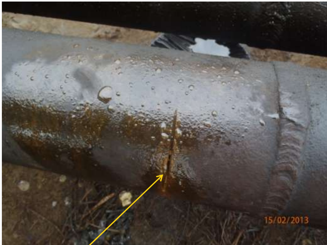
Close up: Hacksaw cut on Obigbo Well 9L flowline at Umuebulu. Picture was taken during Joint Investigation of 15 th February 2013.
