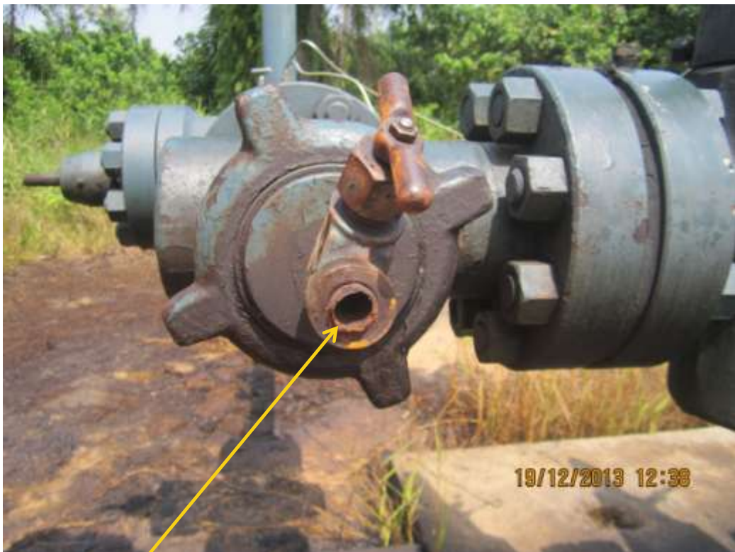
Close-up: Crude oil theft point on Ubie Well4S Wellhead at Idukepuye. Picture was taken during Joint Investigation of 19th December 2013.
