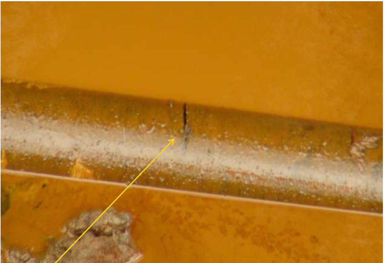
Close-up: Hacksaw cut on Cawthorne Channel 1 Well 49L at Cawthorne Channel. Picture was taken during Joint Investigation of 19th Sept. 2012.
