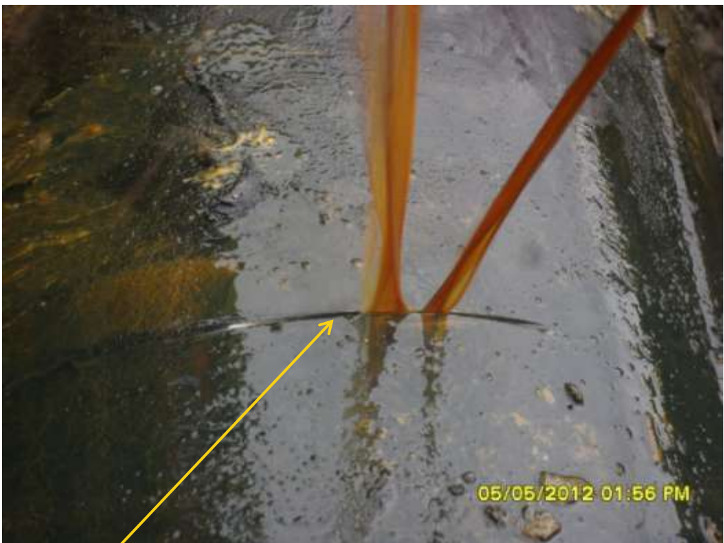
Close up: Hacksaw cut on 16" Nun River – Kolocreek pipeline at Aguobiri. Picture was taken during Joint Investigation of 5 th May 2012.
