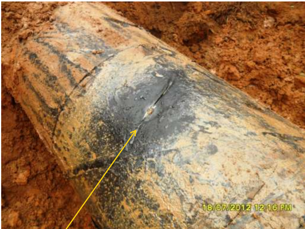
Close up: Hacksaw cut on 18" Assa-Rumuekpe pipeline at Egbeda. Picture was taken during Joint Investigation of 18 th July 2012.
