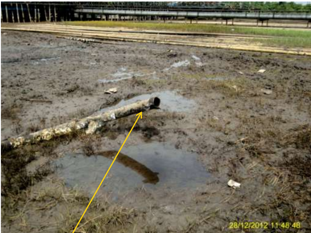
Close up: Ruptured flowline on Nembe1 Well3S flowline at Ewelesuo. Picture was taken during Joint Investigation of 28 th December 2012.
