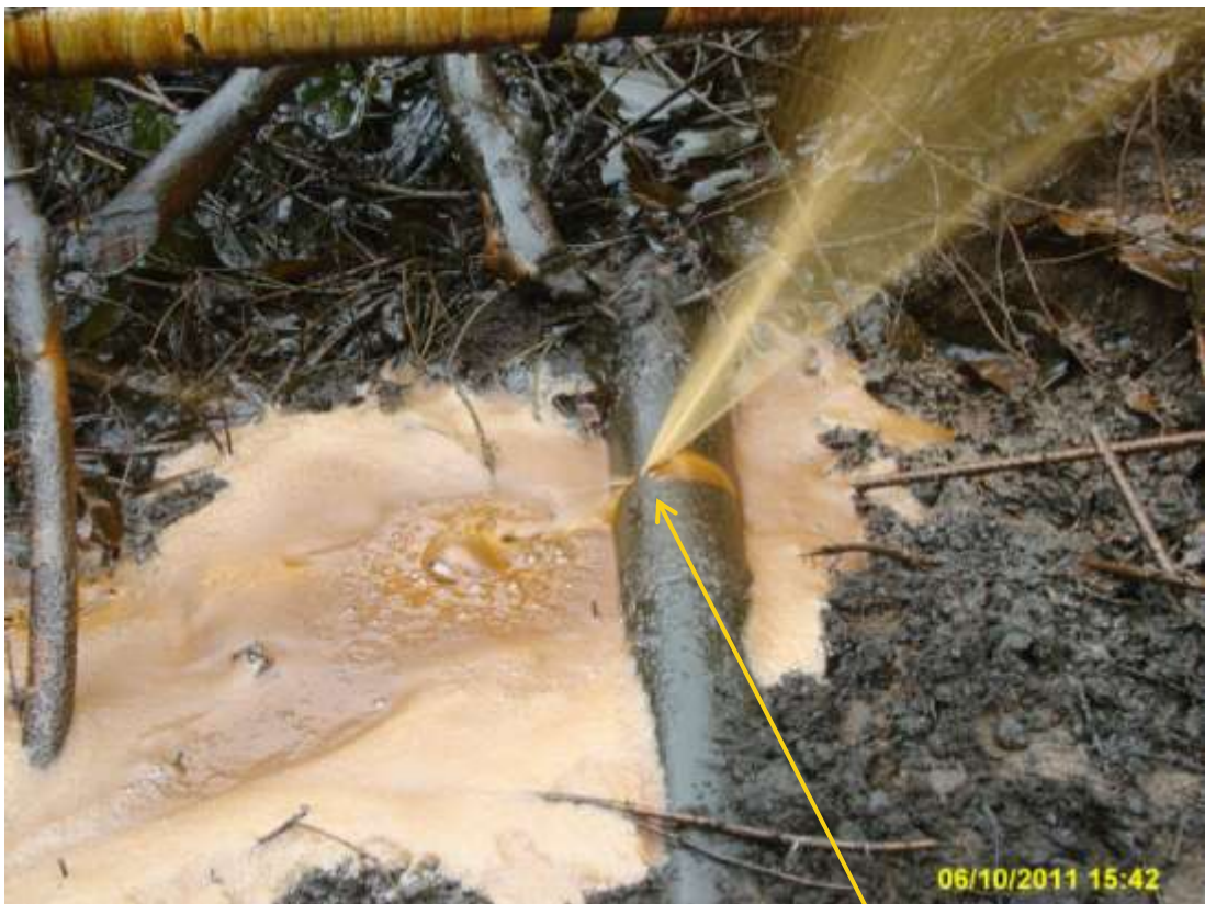
Close-up: Spill due hacksaw cut on 4" ImoRiver1 Well30S flowline at Igiriukwu. Picture taken during Joint Investigation of 6 th October, 2011.
