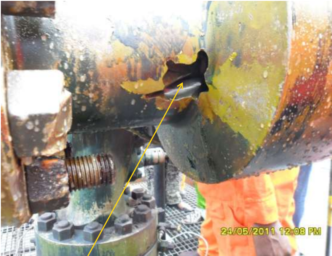
Close-up: Ruptured Bean Box on Nembe Well 20L Well Head in Nembe Creek. Picture was taken during JIV of 24 th May, 2011
