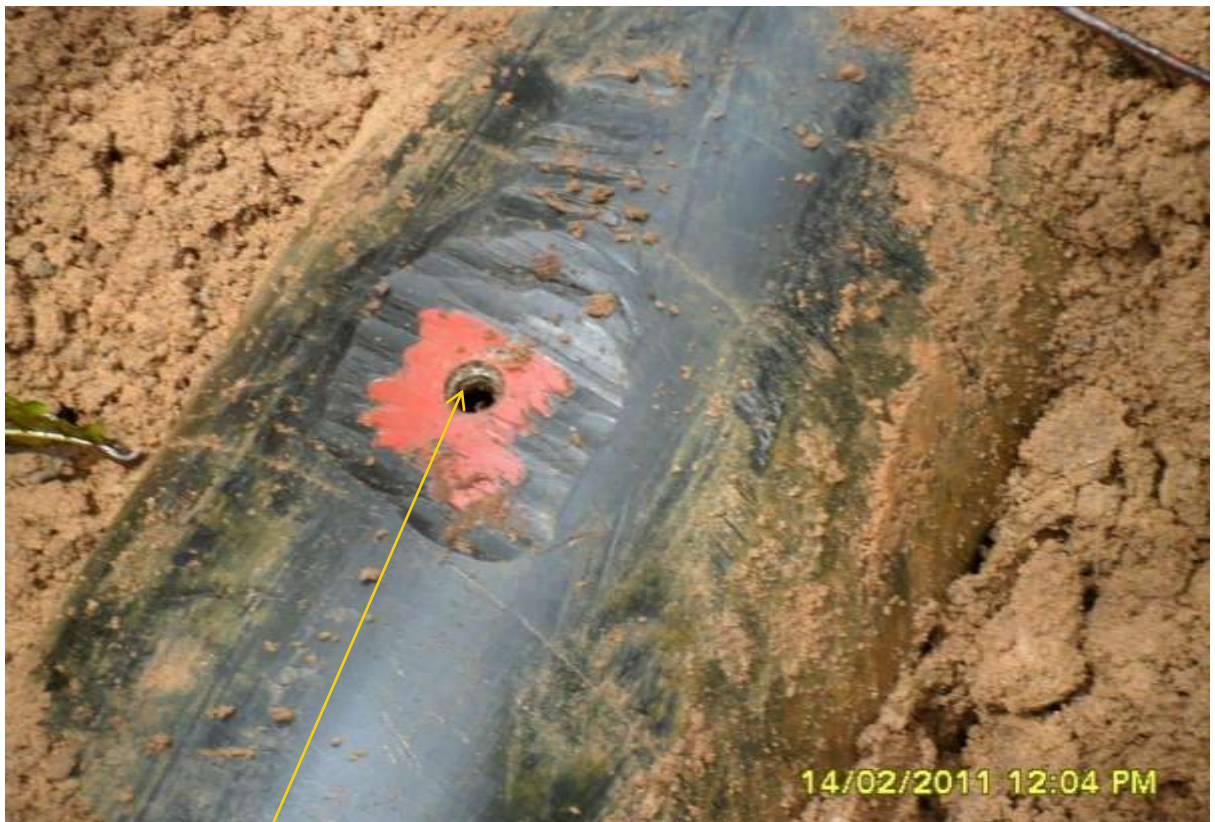
Close-up: Spill due to illegally drilled hole on Imo River well 37L flow line at Owaza. Picture taken during Joint Investigation of 14 th February, 2011.
