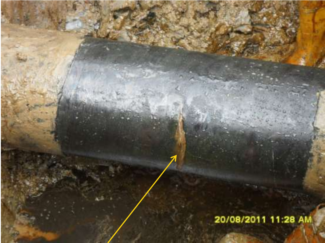
Close-up: Spill due to hacksaw cut on 14in Okordia-Rumuekpe pipeline at Ikarama. Picture taken during Joint Investigation of 19 th August, 2011.
