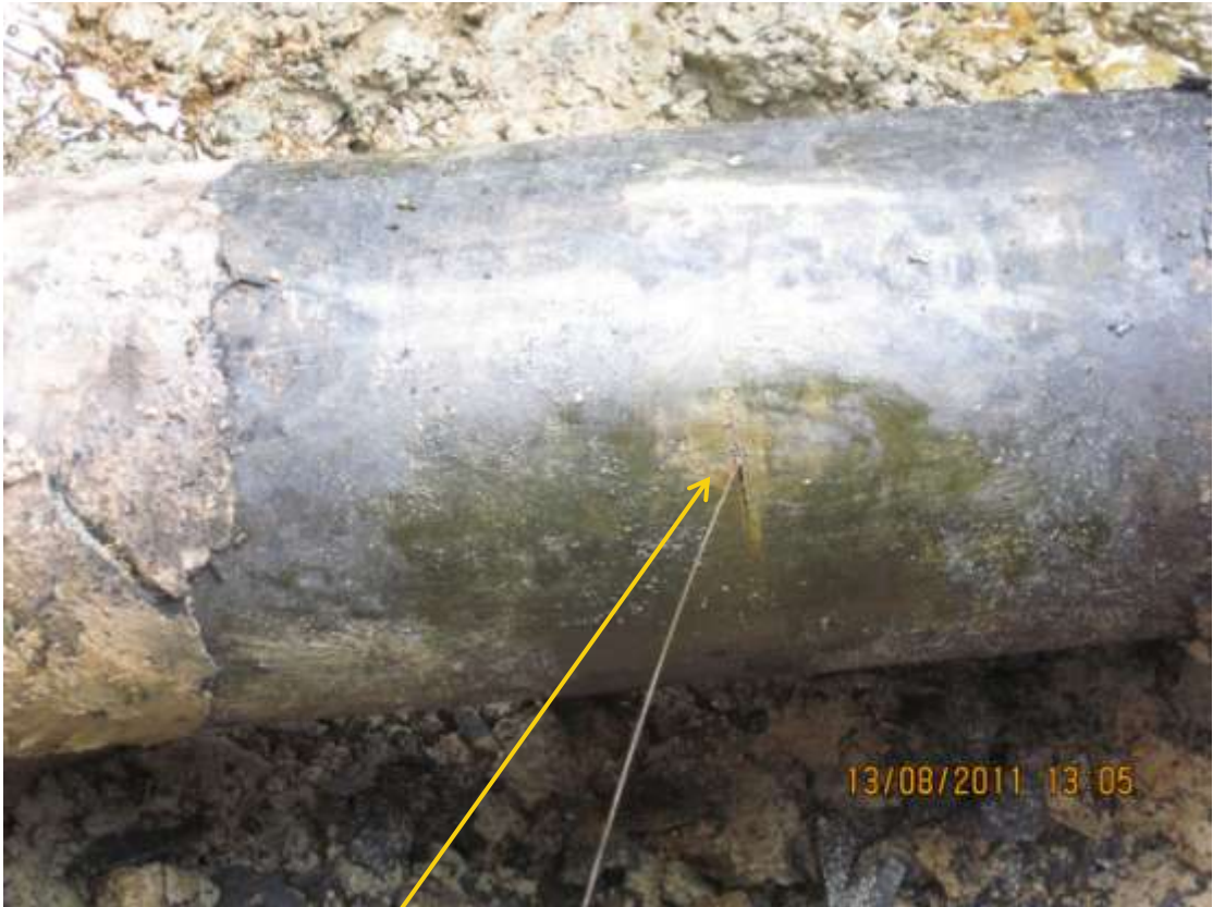
Close-up: Spill due to hacksaw cut on 14" Okordia-Rumuekpe pipeline at Ikarama. Picture taken during Joint Investigation of 13 th August, 2011.
