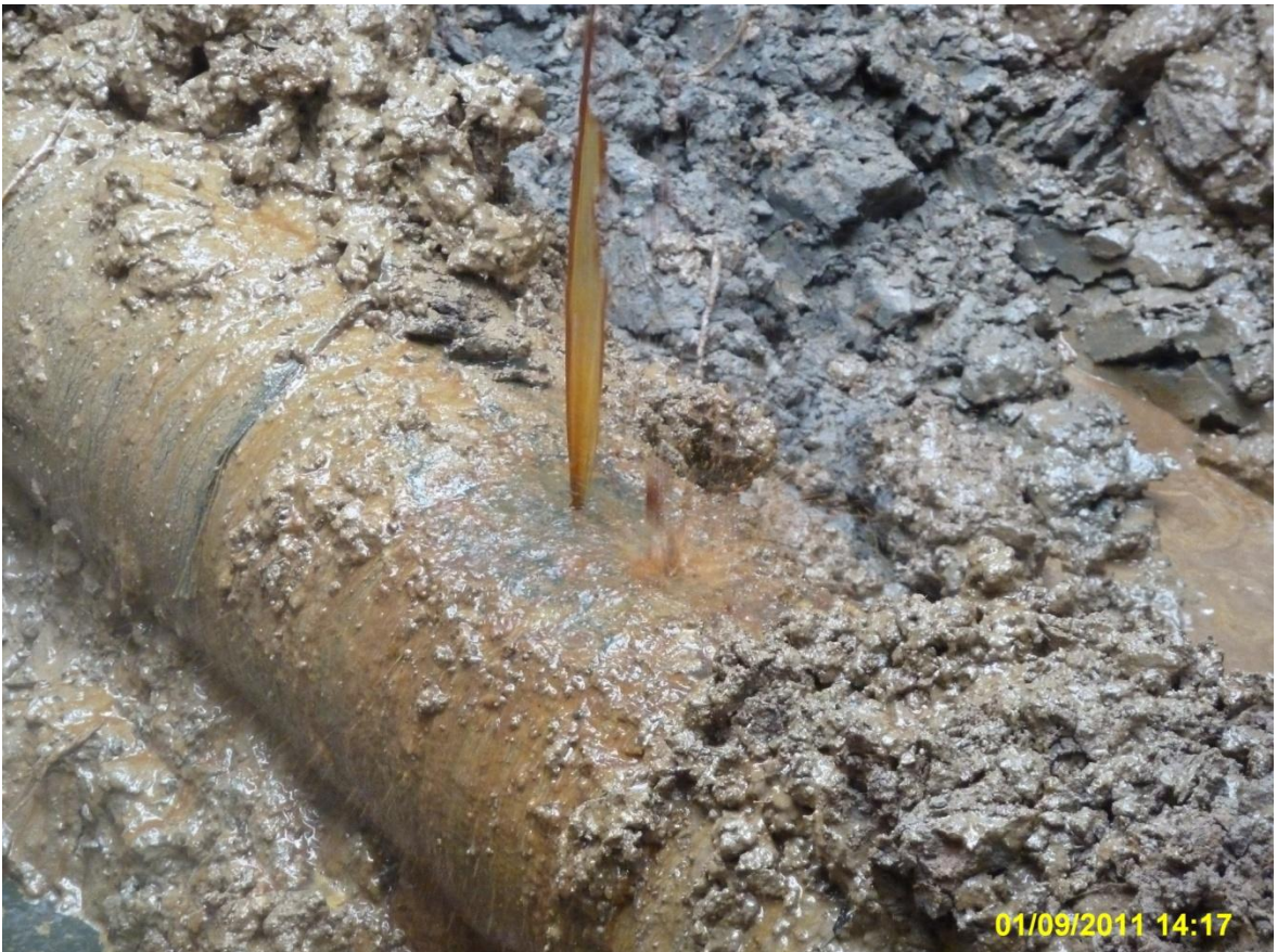
Close-up: Spill due to drilled hole on 10'' Diebu creek-Nun River Pipeline at Oporoma. Picture taken during Joint Investigation of 1 st September, 2011
