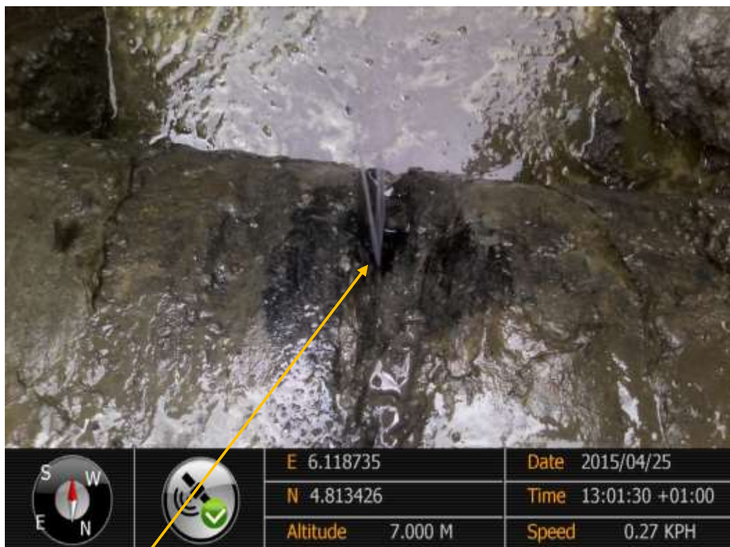
Close-up: Hacksaw Cut on 16" Nun River - Kolo Creek Pipeline at Oporoma. Picture was taken during Joint Investigation of 25 th April 2015.
