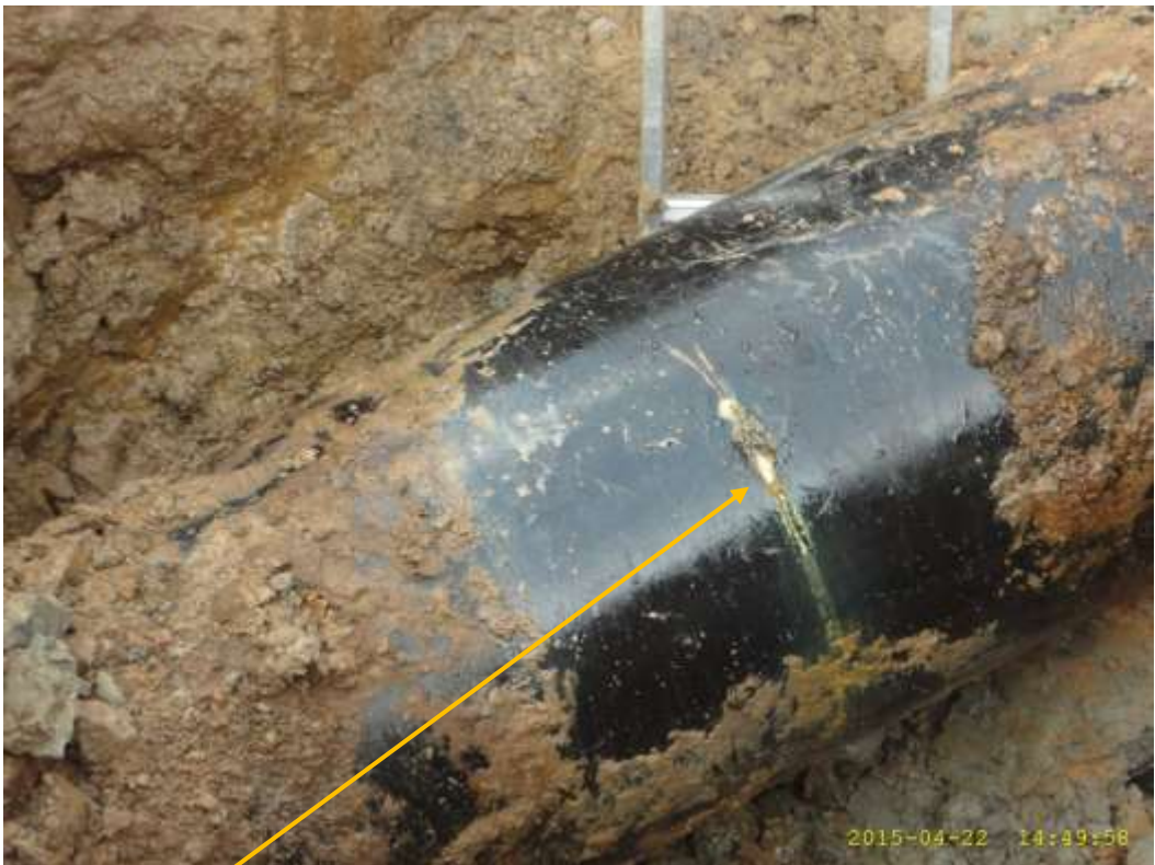
Close-up: Hacksaw Cut on 20" Kolo Creek – Rumuekpe Pipeline at Oruma. Picture was taken during Joint Investigation of 22 nd of April 2015.
