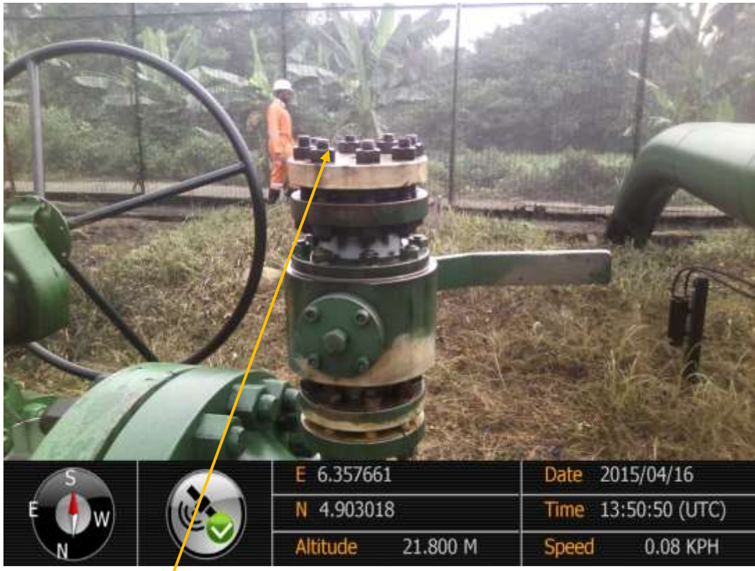
Close-up: Former Location of missing Cork Valve Gauge (2) on Kolocreek Manifold at Otusega. Picture was taken during Joint Investigation of 16 th of April 2015.
